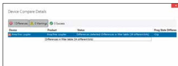
Extensions for ETS support the realisation of professional projects. The ETS App “Project Compare” for instance can be used to compare the actual status of an existing installation with the target status of the ETS project.
